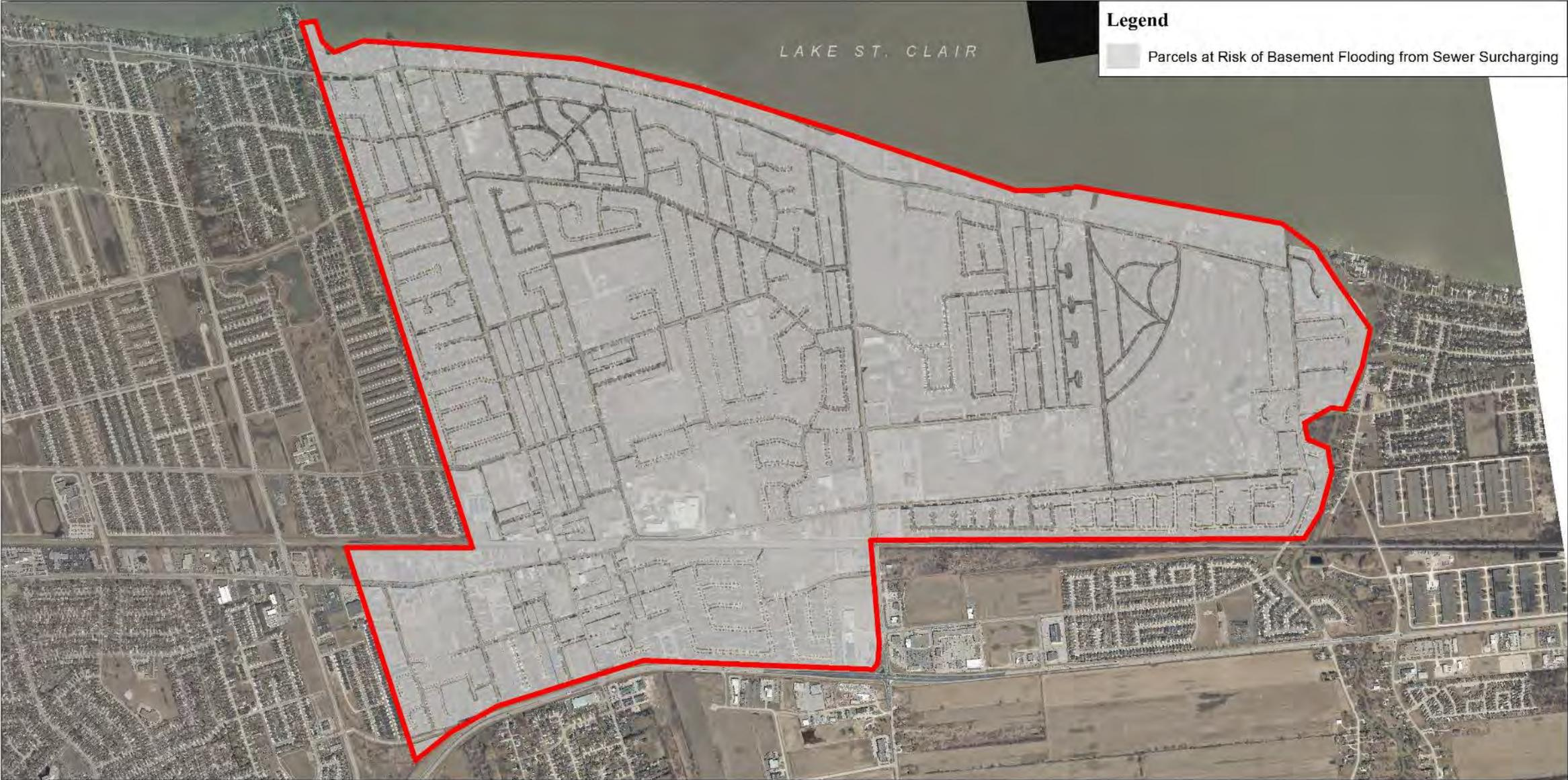
**Zone of Potential Basement Flooding from Sewer Surcharging during a Coastal Flood**
