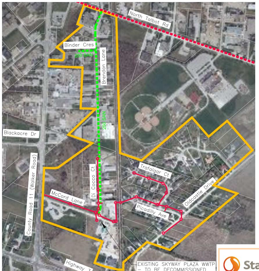
EXISTING SANITARY SEWER EXISTING TRUNK SANITARY SEWER PROPOSED SANITARY SEWER SERVICE AREA BOUNDARY FOR PROPOSED SANITARY SEWER
