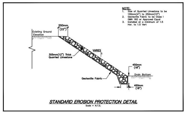
Figure 2 - Standard Erosion Protection Detail
