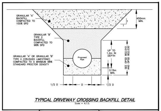
Figure 2- Typical Driveway Crossing Backfill Detail
