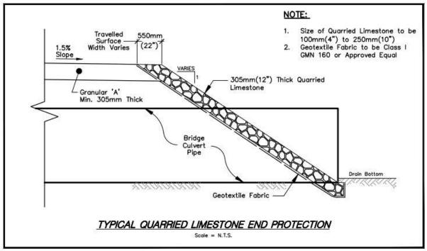
*Figure 4 – Typical Quarried Limestone End Protection*
