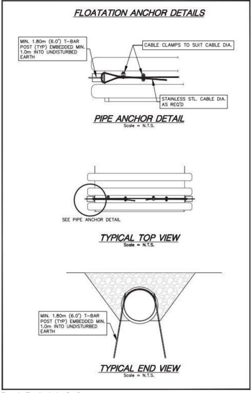
Figure 1 – Flotation Anchor Details
