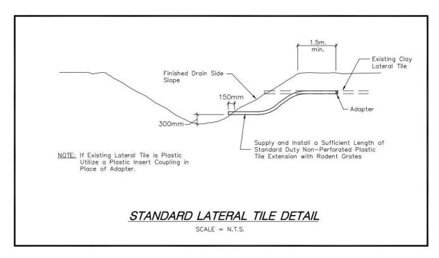
*Figure 8– Standard Lateral Tile Detail*
