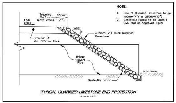
Figure 3 - Typical Quarried Limestone End Protection Detail
