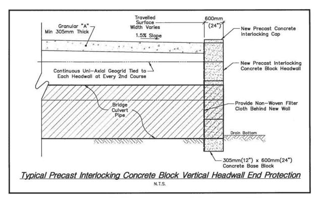
Figure 5– Typical Precast Interlocking Concrete Block Vertical Headwall End Protection
