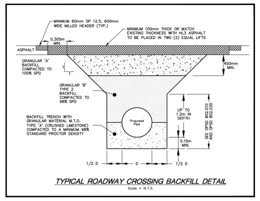
Figure 3 – Typical Roadway Crossing Backfill Detail
