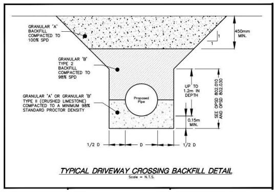
*Figure 2 – Typical Driveway Crossing Backfill Detail*
