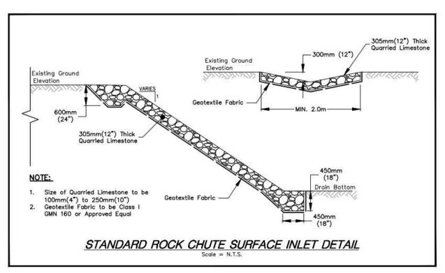
Figure 3 - Standard Rock Chute Surface Inlet Detail
