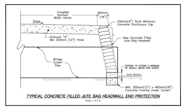
Figure 7– Typical Concrete Filled Jute Bag Headwall End Protection
