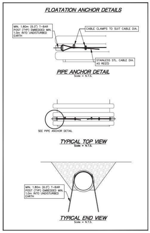
Figure 1 - Flotation Anchor Details
