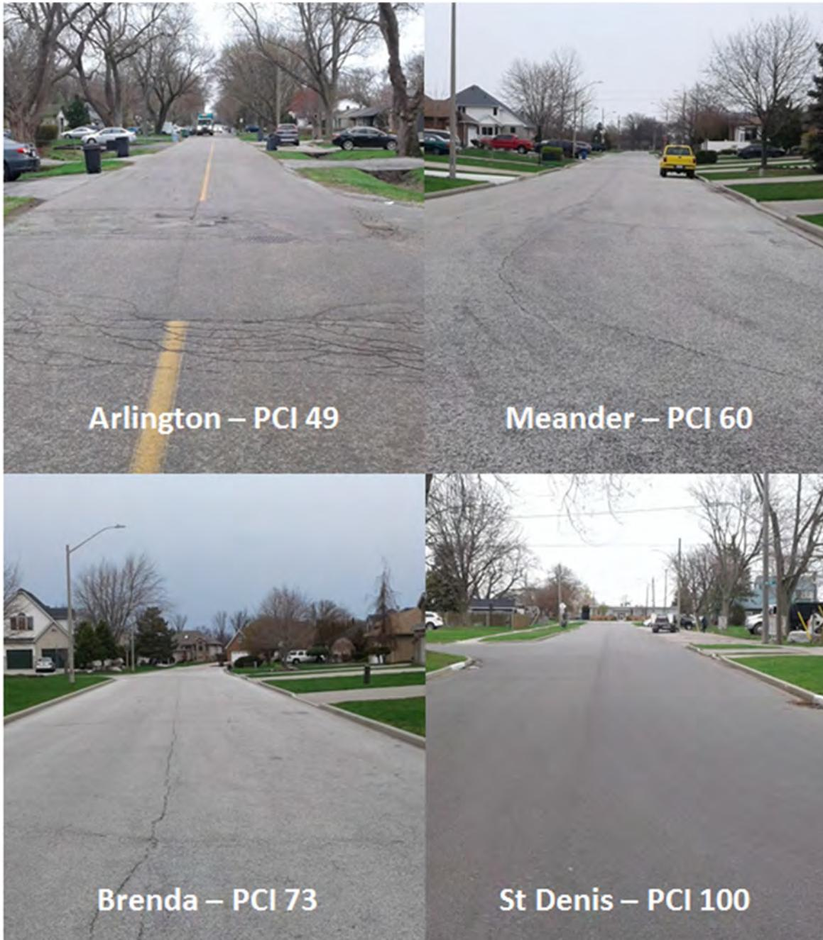
Figure 3-5: Examples of various 2014 PCI ratings
