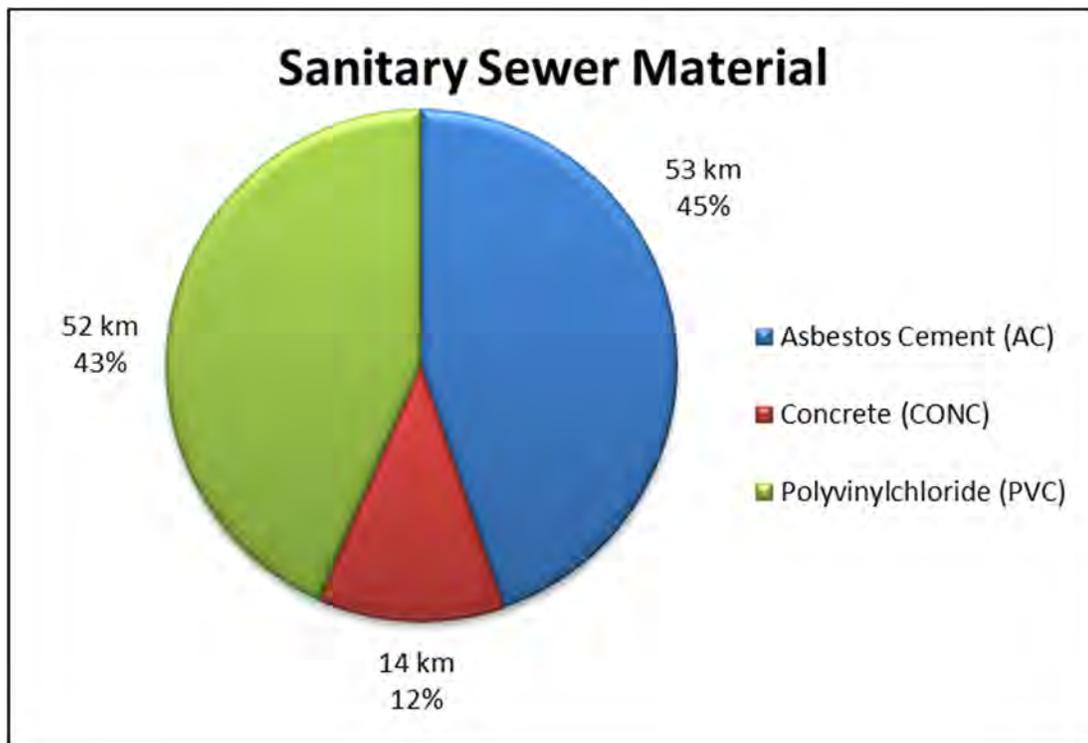
Figure 8-1: Sanitary Sewer Inventory by Material
