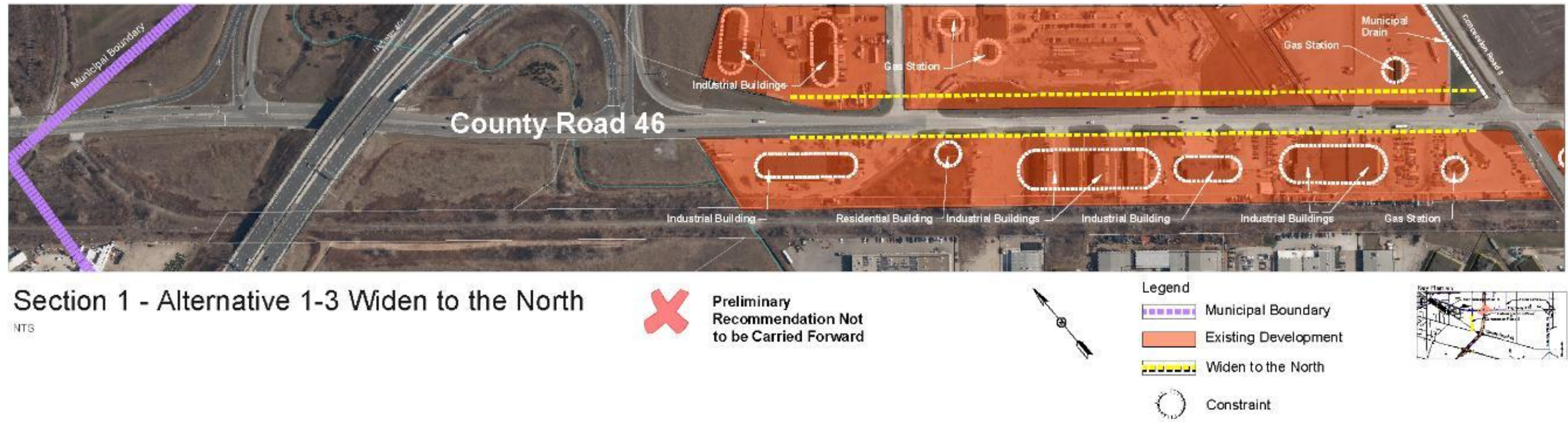
Figure 19: County Road 46 Section 1 Alignment Alternative 1-3
