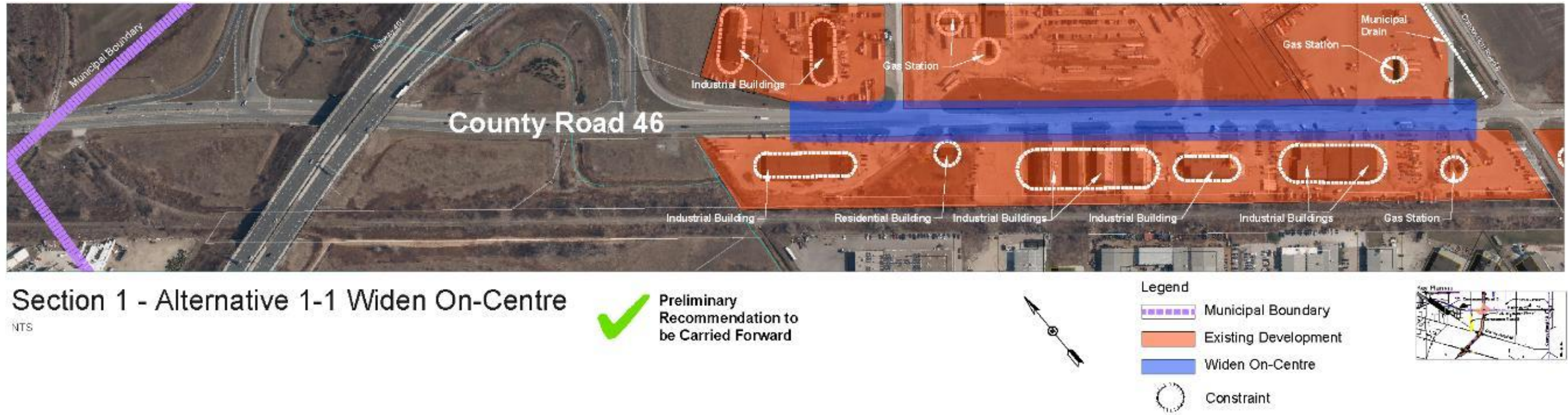
Figure 17: County Road 46 Section 1 Alignment Alternative 1-1
