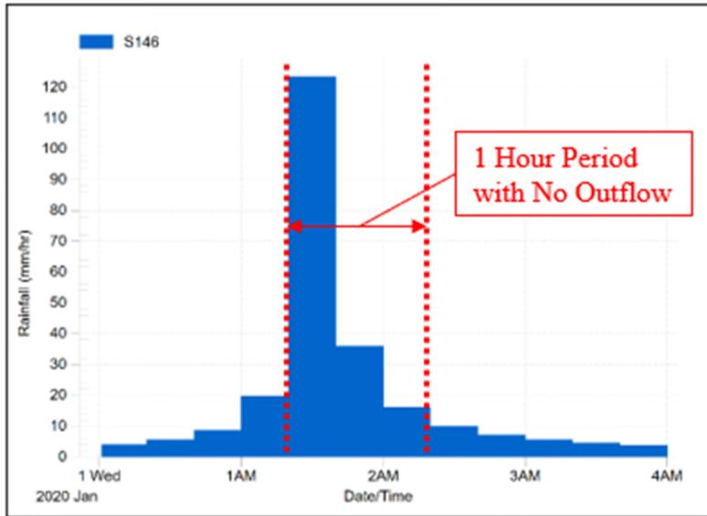
The additional storage volume for the Stress Test is estimated using the same approach and parameters as described in the foregoing SWM – Normal section, with one exception being a conductivity (k) value of 3.0 mm/hr in lieu of 1.0 mm/hr. Graph 5 below represents the difference between the storage volume calculated for the 100-year and Stress Test design storms (i.e., the additional storage volume required over and above the 100-year storage requirements).
