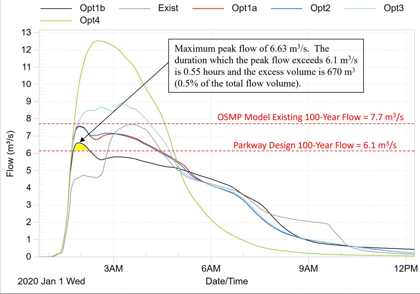
It should be acknowledged that the Wolfe Drain downstream of the study area (i.e., from Highway 401 to Howard Avenue) includes of a relatively wide floodplain as well as a stormwater pond at the northeast corner of Howard Avenue and Highway 401. Thus, the marginal excess volume can reasonably be expected to have no adverse impact on the downstream receivers.
