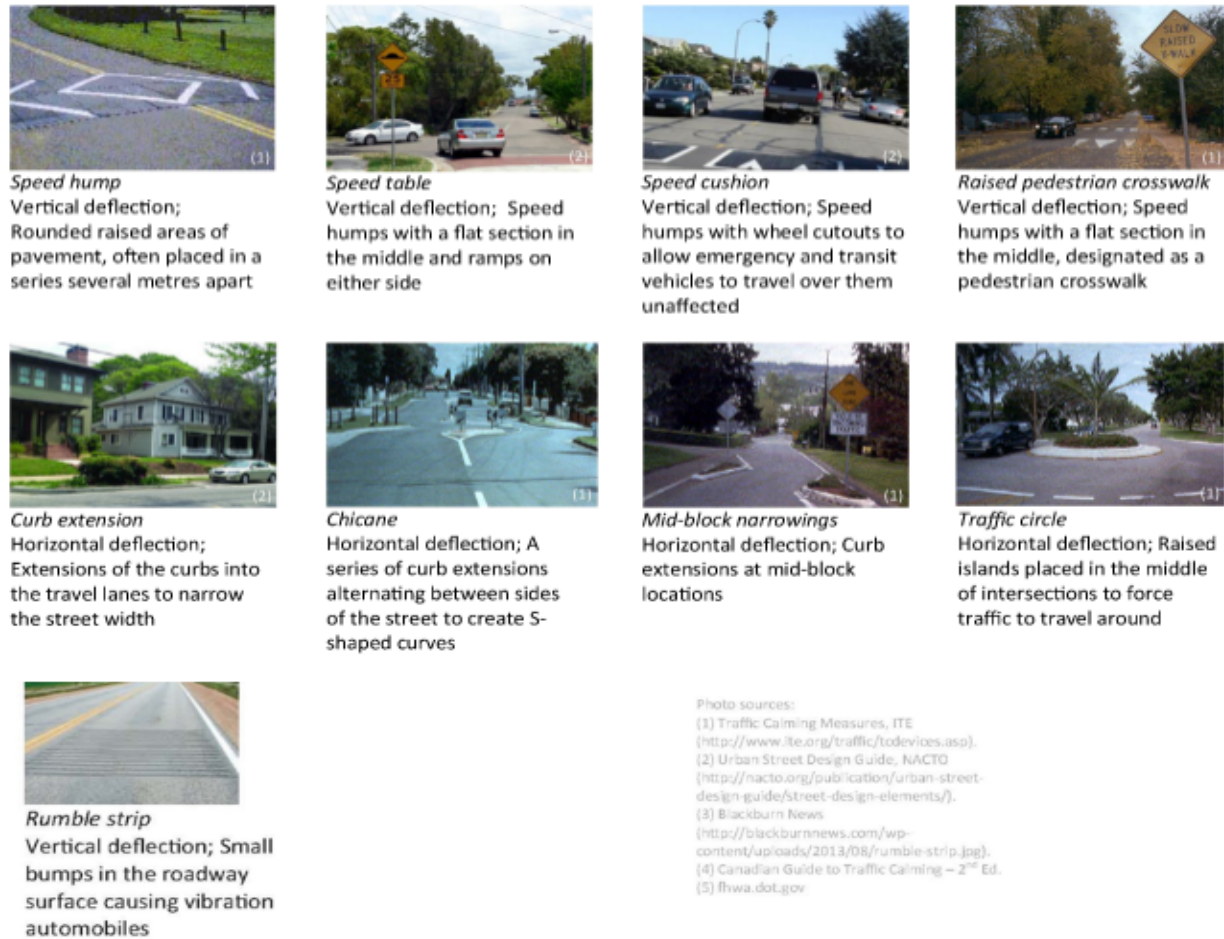
Figure 3 - Traffic Calming Measures by Road Classification
